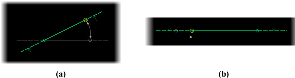
Figure 290 – Interactive rotating with Perpendicular option turned off – rotation (a), changing the rotation center (b)
