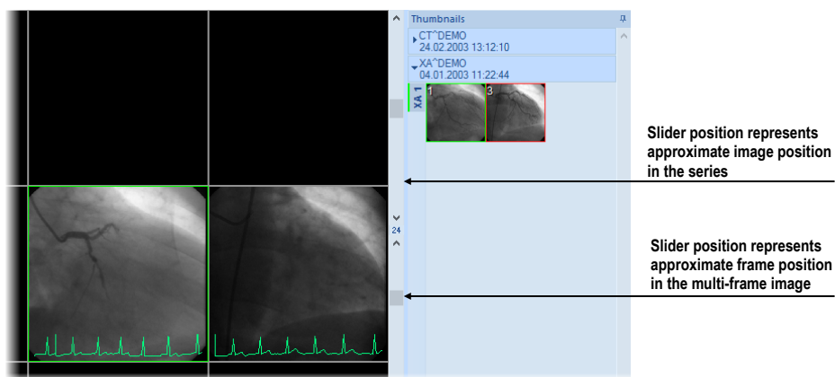
Figure 130 – Working area with multiframe image in current view
