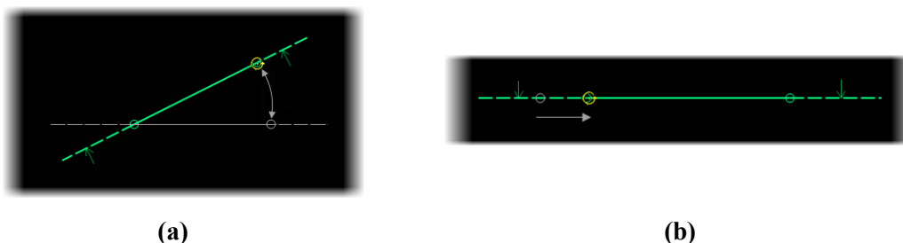
Figure 299 – Interactive rotating, Perpendicular option is off, a) section line rotation, b) changing the rotation center
